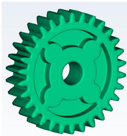
Figure 1: Spur gear model with 2 module and 30 teeth configuration
